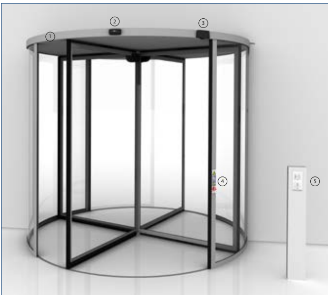
1= revolving door drive (can alternatively be installed in the floor) | 2 = radar movement detector | 3 = active infrared detector | 4 = emergency stop push button | 5 = programme switch with key switch (bollard on-site)
